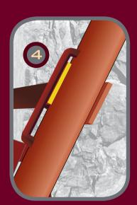
INSTALL CAMLOK PROPS MAX 1.5M APART CENTRE TO CENTRE AND MIN 1.5M OR 1.0M FROM FACE DEPENDENT ON CANOPY SIZE
